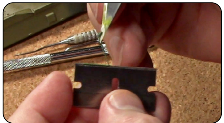
Carefully lift the strap material off the razor blade with a hobby knife blade.
