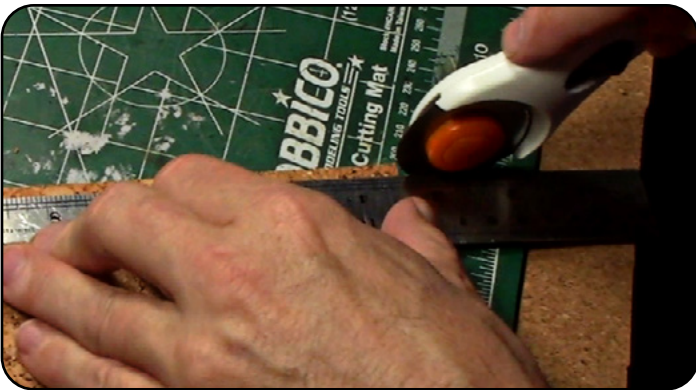
Using a straightedge (ruler) and a rotary cutter also works well.
